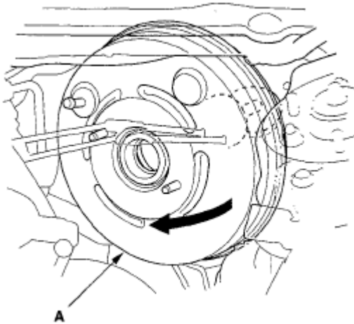
Fig. 44: Twisting Brake Booster
