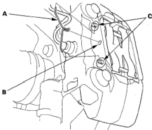
Fig. 20: Identifying Calliper Hole And Clip Courtesy of AMERICAN HONDA MOTOR CO., INC.
